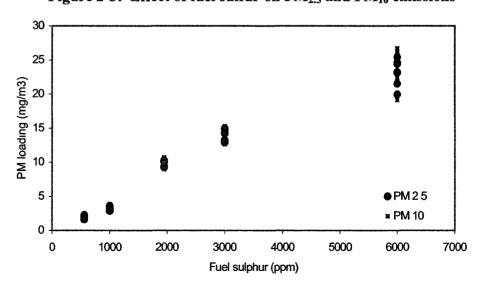
Figure 2-3: Effect of fuel sulfur on PM<sub>2.5</sub> and PM<sub>10</sub> emissions
