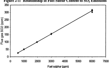
Figure 2-1: Relationship of Fuel Sulfur Content to SO<sub>2</sub> Emissions
