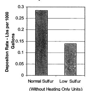
Figure 3-2: Measured Boiler Deposits - Normal and Low Sulfur Fuel Oil
